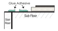
Line the Flush Stairnose up with the edges of the Stair and place the inside against the outside of the Stair Riser.
