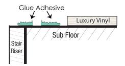
Line the Overlap Stairnose up with the edges of the Stair and place the inside against the outside of the Stair Riser.
